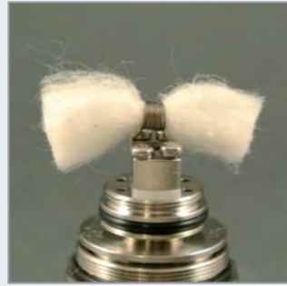
Standard-Microcoil, 0.32 Kanthal / 7 Windungen / Ø3.0 mm / KoGenDo-Watte / ca. 2 Ω
