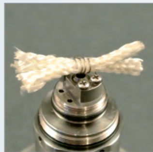
Standard-Faser-Coil / 0.3 Kanthal / 4 Windungen / Ø ca. 5 mm / 3 mm Braided Cord (doppelt) / ca. 1,0 Ω
