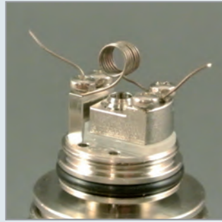
Standard-Microcoil, 0.32 Kanthal / 7 Windungen / Ø3.0 mm / KoGenDo-Watte / ca. 2 Ω
