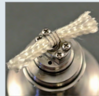
Standard-Faser-Coil / 0.3 Kanthal / 4 Windungen / Ø ca. 5 mm / 3 mm Braided Cord (doppelt) / ca. 1,0 Ω
