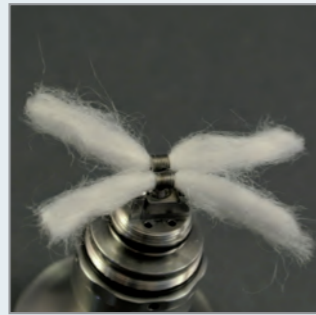
Dual-Microcoil / 0.28 Kanthal / 2 x 9 Windungen / Ø2.5 mm / Blackwool / ca. 0,8 Ω
