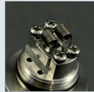
Dual-Microcoil / 0.28 Kanthal / 2 x 9 Windungen / Ø2.5 mm / Blackwool / ca. 0,8 Ω
